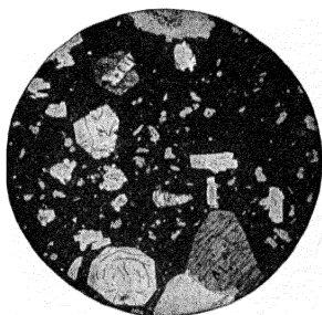
FIG. 113.—Microscopic section of Vesuvian lava, containing crystals of felspar, augite, and leucite in a black glass (about \frac{1}{2} ).
